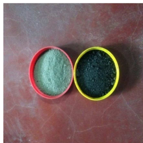
Figure 4. Raw sample (at the left) & Biochar (at the right).
